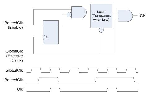
This diagram shows that the resulting clock occurs synchronous to the global clock on the first clock after a rising edge of the routed clock.
