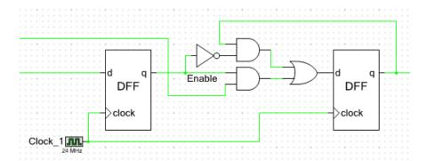
If access to a clock is needed, for example to generate a clock to send to a pin, then a 2x clock should be used to clock a toggle flip-flop. The output of that flip-flop can then be used with the associated timing analysis available.
