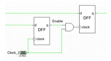
This circuit is implemented with a routed clock, has no timing analysis support, and is prone to the generation of glitches on the clock signal when the clock is enabled and disabled.
