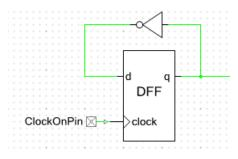
If input synchronization was not enabled at the pin, there would not be a global clock to use to transform the routed clock, and the routed clock would be used directly.
