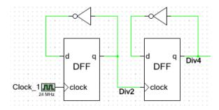
The report file indicates that one global clock has been used and that the single routed clock has been transformed using the global clock as the effective clock.
