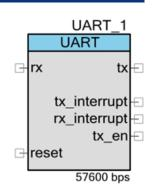
Component provides configuration support for the number of data bits, stop bits, parity, hardware flow control, and parity generation and detection.
