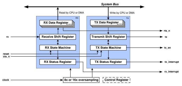
The UART Component provides synchronous communication commonly referred to as RS232 or RS485. The UART can be configured for full duplex, half duplex, RX only, or TX only operation. The following sections give an overview of how to use the UART Component.
