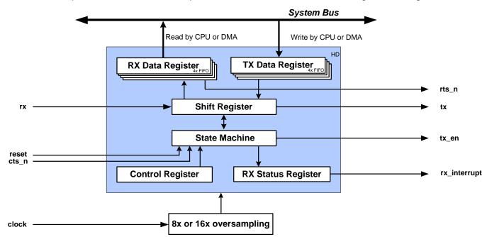
This mode implements a full UART, but uses half as many resources as the full UART configuration. In this configuration, the UART can be configured to switch between RX mode and TX mode, but cannot perform RX and TX operations simultaneously. The RX or TX configuration can be loaded by calling the UART\_LoadRxConfig() or UART\_LoadTxConfig() function.
